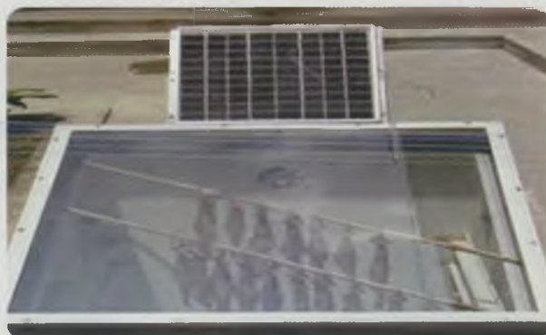
Fish processing on solar drier under AICRP on Post-harvest technology, F/ Fishery Sciences
